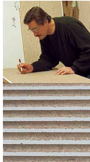
Some bits cut very cleanly. There's virtually no chipout on this panel.
